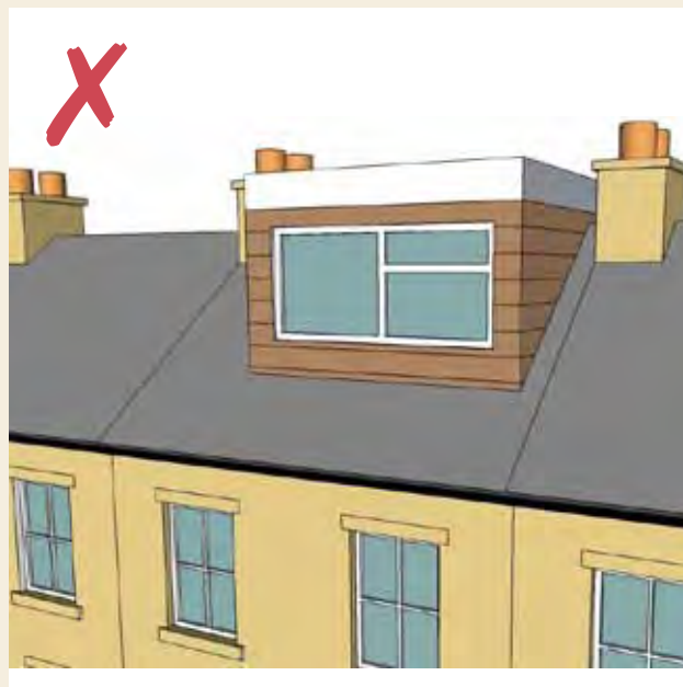
Figure 44: Unacceptable – above ridge, too large, poor materials, poor window details
