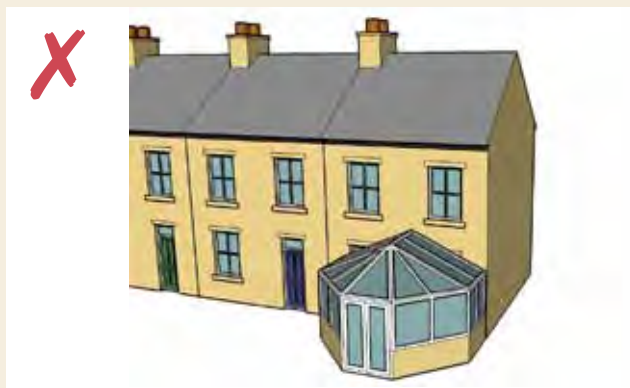
Figure 22: Conservatory not acceptable to front of house
