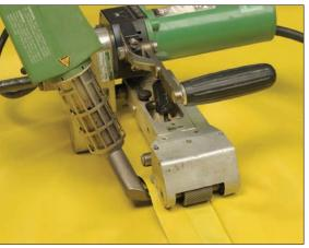
Figure A4.30 Thermal welding technique (courtesy Industrial Textiles & Plastics Ltd)
