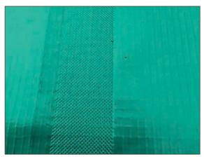
Wedge weld on an LDPE aluminium gas membrane, where the installer used metal nip rollers. This destroyed the top layer and probably the bottom layer, leaving aluminium exposed between the weaves. This failed dielectric testing along all joints (courtesy MEC Environmental Ltd)
