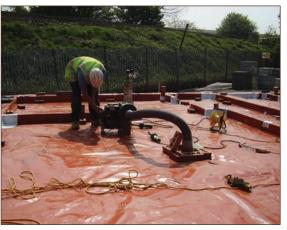
Figure A4.38 Tracer gas testing (courtesy PAGeotechnical Ltd)
