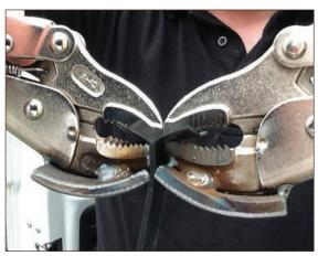
Testing a weld with 'dog bone' grips (courtesy MEC Environmental Ltd)
