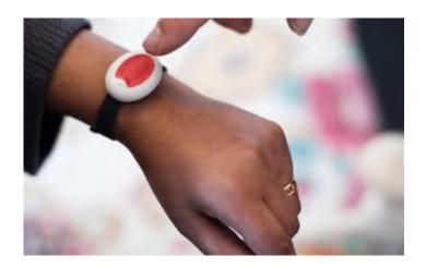
To activate the alarm you simply press the button on your pendant or wristband. The operator will be contacted through the alarm base unit. They will know who you are, where you are and be ready to help and support you.
