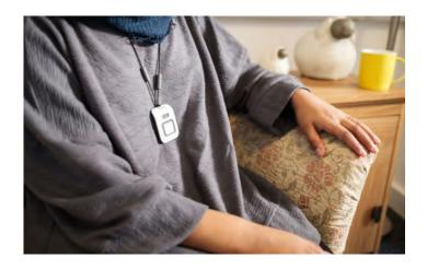
The basic equipment is a control box and pendant. The equipment is connected to your phone line and the pendant is to wear around your neck or wrist.
